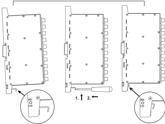
Figure 2. Mounting to DIN rail
