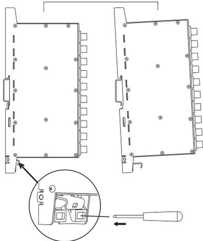
Figure 3. Demounting from DIN rail
