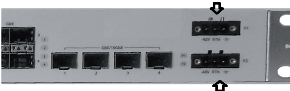
Figure 4-2: OLT chassis redundant power supply input connectors
